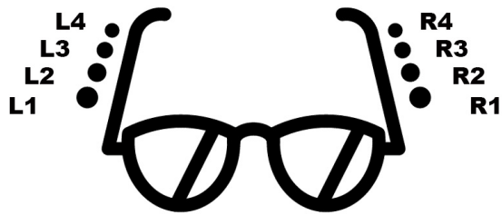
Figure 8. the Third Eye vibration motors allocation.
