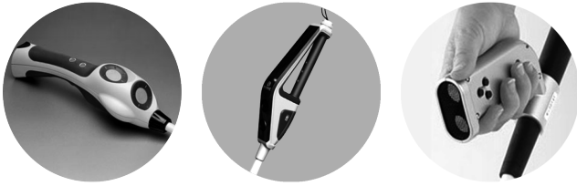
Figure 2. Cane-based Ultrasonic System. (a: UltraCane, b: K-Sonar, c: iSonic)
