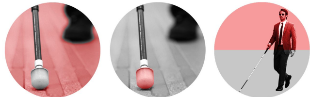
Figure 1. Diagram Showing Drawbacks of White Cane (a: limited to ground level, b: only detects object it touches, c: cannot avoid obstacles over waist level)
